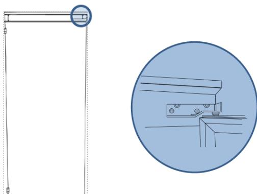
To reverse the door you will need to tilt the appliance backward to access the lower hinge which holds screws. Do not tilt the appliance more than 45 degrees and do not lay the appliance flat on its side.
