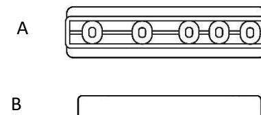
2. Open the cabinet door and the appliance door, mark on the back of the cabinet door where the top of the appliance door reaches. Place the door guide (part A) on the back of the cabinet door, in the location shown below and mark the position of the first hole and the last hole on the door guide. Fix the door guide into place with 2 torx headed screws.
