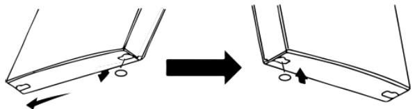
3. Remove all of the screw cap covers on the opposite side of the appliance from where the hinges have just been removed. Remove the hinge plugs on the top and bottom of the door and fix them to the opposite side.
