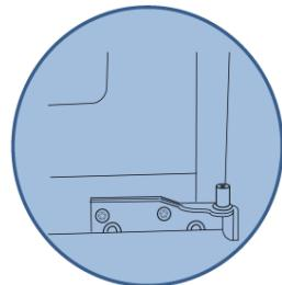
2. Unscrew the 2 screws from the lower hinge and remove the hinge. Do not fix the hinge to the opposite side at this stage.
