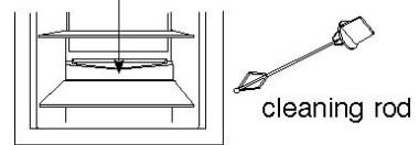
Caution: Always keep the drain over the vegetable and fruit tray clear to ensure the normal flow of defrosted water. Use the rod provided to clear any blockages.
