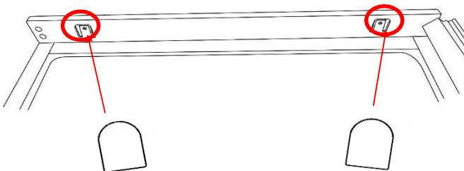
Apply a foot blanking covers by clipping them into place on the feet at the bottom of the appliance. The plastic stem on the foot caps is there as a guide of what the distance between the product and the edge of the cabinet should be (approximately 42mm). Snap off the plastic stem after installation.
