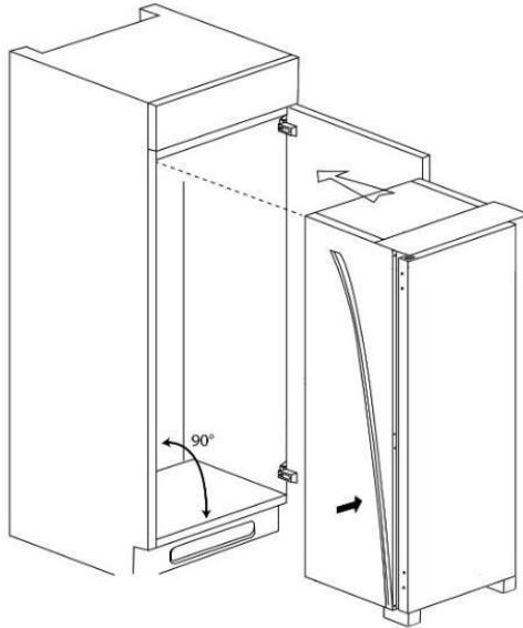
Open the door and push the side of the appliance without the hinges against the side of cabinet wall. Fix the appliance in two places, 1) 2 torx headed screws in the top plinth at the top of the appliance and 2) 2 torx screws in the feet (1 in each foot) at the bottom of the appliance.
