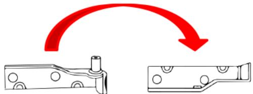
4. Flip over the upper hinge 180° (so the pin is pointing upwards) and fix on to the opposite side at the bottom of the appliance. Place the door back on to the lower hinge.
