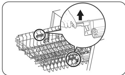
To raise the upper basket, just lift the upper basket at the center of each side until the basket locks into place in the upper position. It is not necessary to lift the adjuster handle. To lower the upper basket, lift the adjust handles on each side to release the basket and lower it to the lower position
