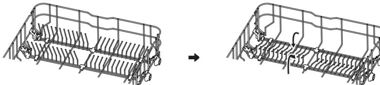
The spikes of the lower basket are used for holding plates and a platter. They can be lowered to make more room for large items.
