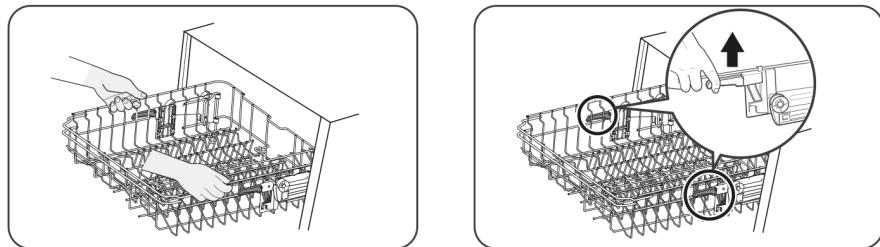
To raise the upper basket, just lift the upper basket at the center of each side until the basket locks into place in the upper position. It is not necessary to lift the adjuster handle. To lower the upper basket, lift the adjust handles on each side to release the basket and lower it to the lower position
