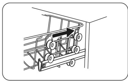
The height of the upper basket can be easily adjusted to accommodate taller dishes in either the upper or lower basket.
