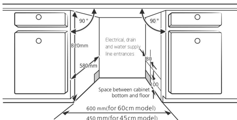
If dishwasher is installed at the corner of the cabinet, there should be some space when the door is opened.
