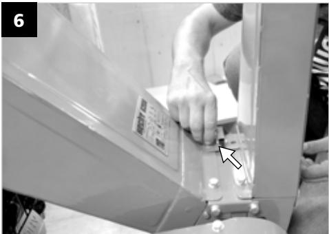
**EN** Install the running safety lock switch (on the cable on the side of the machine) using two screws and tighten properly.
